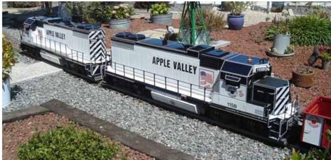
Two GP 38's built by Rail Systems. 18 hp Briggs & Stratton engine with alternator and both units have hydraulic drive. Features an air over hydraulic disc brake system and electric fuel pump. Electronic controller is hand held. The second locomotive is equipped with a Phoenix sound system powered by a 350 watt amp. The first unit can be run without the second unit if desired. These locomotives are highly detailed with a custom paint job. Units can not be sold separately.
