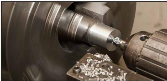
Bored a 0.814” dia hole 0.25” deep for the die and chamfered both edges. Hold the depth of the hole to within a thousandth or two. Both holes should be machined at the same time to ensure concentricity.
