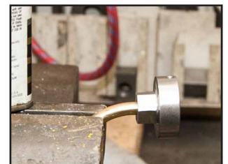
The originals right front, the new ones left front, other holders in the background. They hold the die with the cutting facing outwards and are guided by pins held in the tail-stock.
