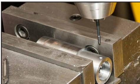
be 0.125” from the bottom of the 0.814” dia. hole. That should help keep the die from being pulled off parallel by the set screw.
