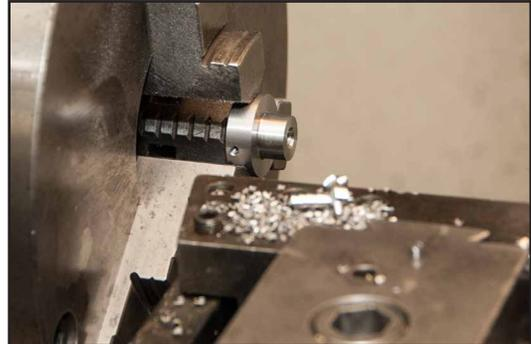
tail-stock to align the part square in the 3 jaw chuck. Basically the tail-stock was brought up to the part and the part held tight against the face of the chuck in the tail-stock and then the 3 jaw is tightened. This holds the part square enough for this operation.
